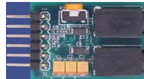
14.4.1. Picture on the left: Digilent PModSF 2 Megabyte flash memory module; Picture on the right: Digilent PmodAMP1 Speaker/Headphone amplifier module to boost the audio signal strength.
