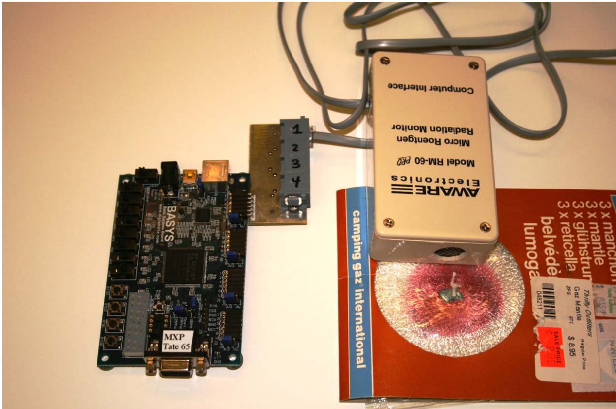
Figure 13.4. RM 60 Radiation Monitor with Thorium Oxide gas mantel and BASYS board. The RM 60 has been connected to pin 1 of the BASYS board's JA edge connector which corresponds to pin P81 on the FPGA.
