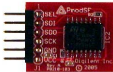
14.4.1. Picture on the left: Digilent PModSF 2 Megabyte flash memory module; Picture on the right: Digilent PmodAMP1 Speaker/Headphone amplifier module to boost the audio signal strength.
